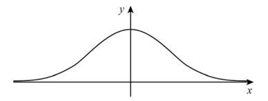
The graph is formed from two convex sections, where the gradient is increasing, and one concave section, where the gradient is decreasing.
